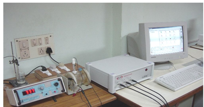
Fig 4 Potentio dynamic polarization Experiment set up
