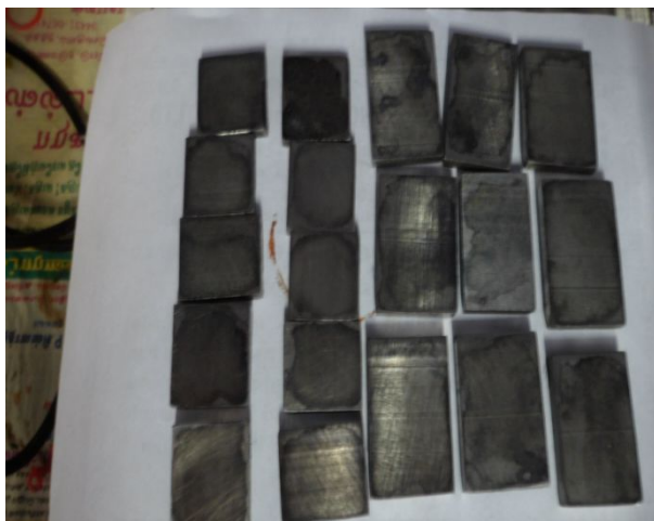
Fig 2 Nano coated carbon steel plates using solution casting method
